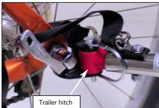
**You may need to adjust the bike hitch to align the holes with the hole in the trailer hitch. Align holes, slide through, then close tab-lock pin.**
