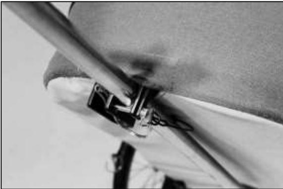
**6. Secure tow bar in front foot with tab lock pin. Lock pin in place with wire.**
