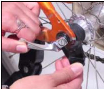
2. **Adjust nut to produce the proper resistance while rotating the quick release level forward.**
