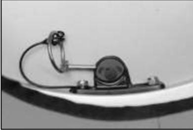
**1. Remove pin from inside trailer foot well.**
