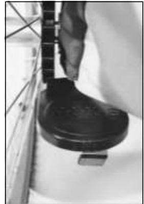
Check that the sprocket is completely engaged on hub. Use a screwdriver if needed. Insert axle into receiver hole, make sure that brake pedal is up. Pedal actuator should engage sprocket when brake is applied.
