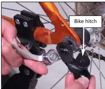
1. **Rotate skewer arm and loosen nut on chain side of bicycle. Remove skewer from axle and then replace it with bike hitch at dropout. Replace spring and nut on chain side of bicycle and tighten.**
